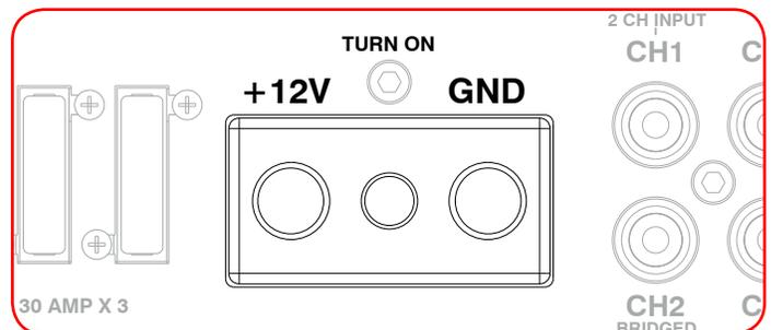
The Turn On input should be connected to the amplifier +12V DC remote turn-on output of your after-market source unit. In most cases this is a blue wire with a white stripe. Note: On some source units, there are power antenna AND remote turn-on wires. If you only hear audio when listening to the AM/FM tuner, your amp may be connected to the wrong wire.
